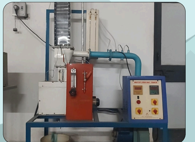
Water Cooling Tower
