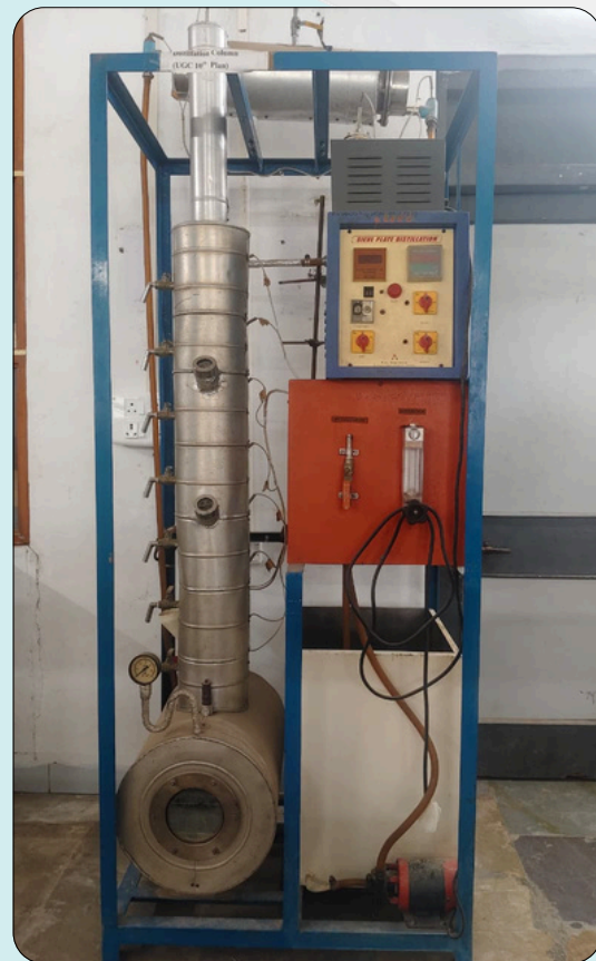
Silver Plate Distillation Column
